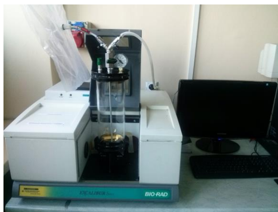
Fig. 1. The view of the position of the test gases by FTIR
