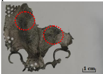
Fig. 1. Cast of a frame bracket prosthesis with a visible casting defect in the form of blisters
