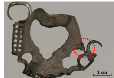
Fig. 3. Frame prosthesis with a visible cold fracture on the side of the bracket
