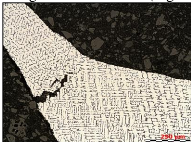
Fig. 4. Microstructure of the Co-Cr-Mo alloy with a visible casting defect – intercrystalline crack
